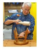
before the glue dries to tease the spindles and stretchers into alignment so that the stool doesn't wobble!
